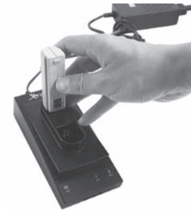
Figure 14: Battery Charger with Battery.
