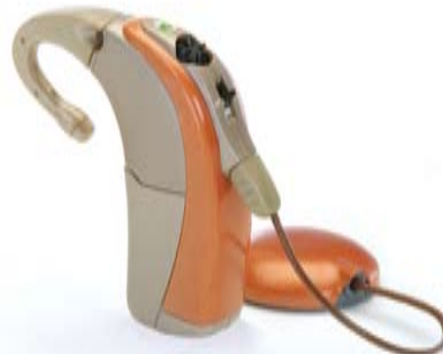
Figure 1. The Harmony BTE sound processor with the small T-Mic ® attached.
