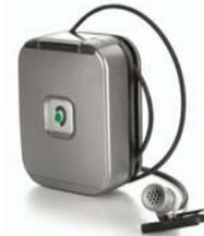
2. Ensure that the FM system is functioning appropriately by listening to the FM system through an amplified speaker or walkman-style earphones.
