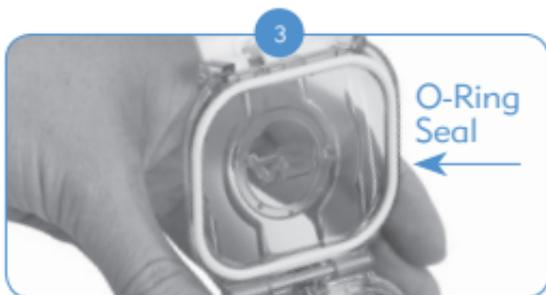
Before placing the Naída CI in the AquaCase, visually inspect the O-Ring seal to make sure it is placed correctly. **Visually confirm that the O-Ring is not dry, brittle or dirty. If it is, replace O-Ring prior to use.**
