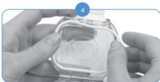
While holding the O-Ring in the groove with one hand, carefully stretch the remaining portion of the O-Ring into the remaining groove.
