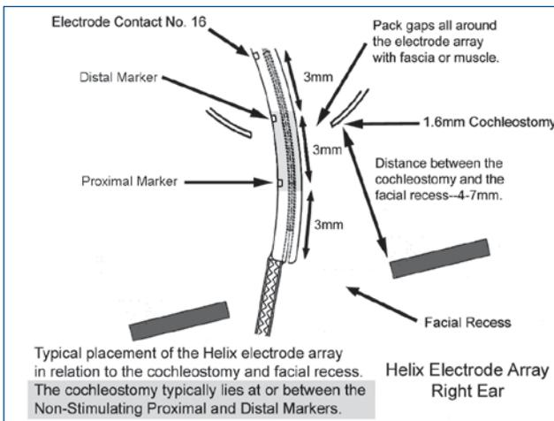
Figure 1. Relative position of the inserted HiFocus Ij Electrode following a typical insertion
