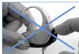
FIGURE 6: Removal of HiRes Auria Processor Accent Color Cover
