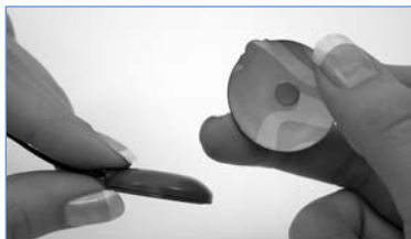
FIGURE 5: Removal of Auria Accent Color Headpiece Cap
