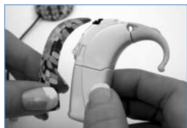
FIGURE 6: Removal of HiRes Auria Processor Accent Color Cover
