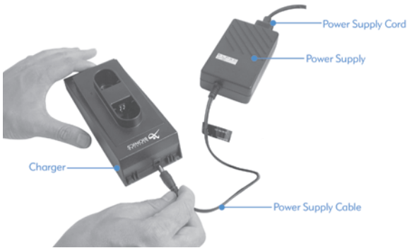
Figure 13: Connecting the Power Supply to the Charger.
